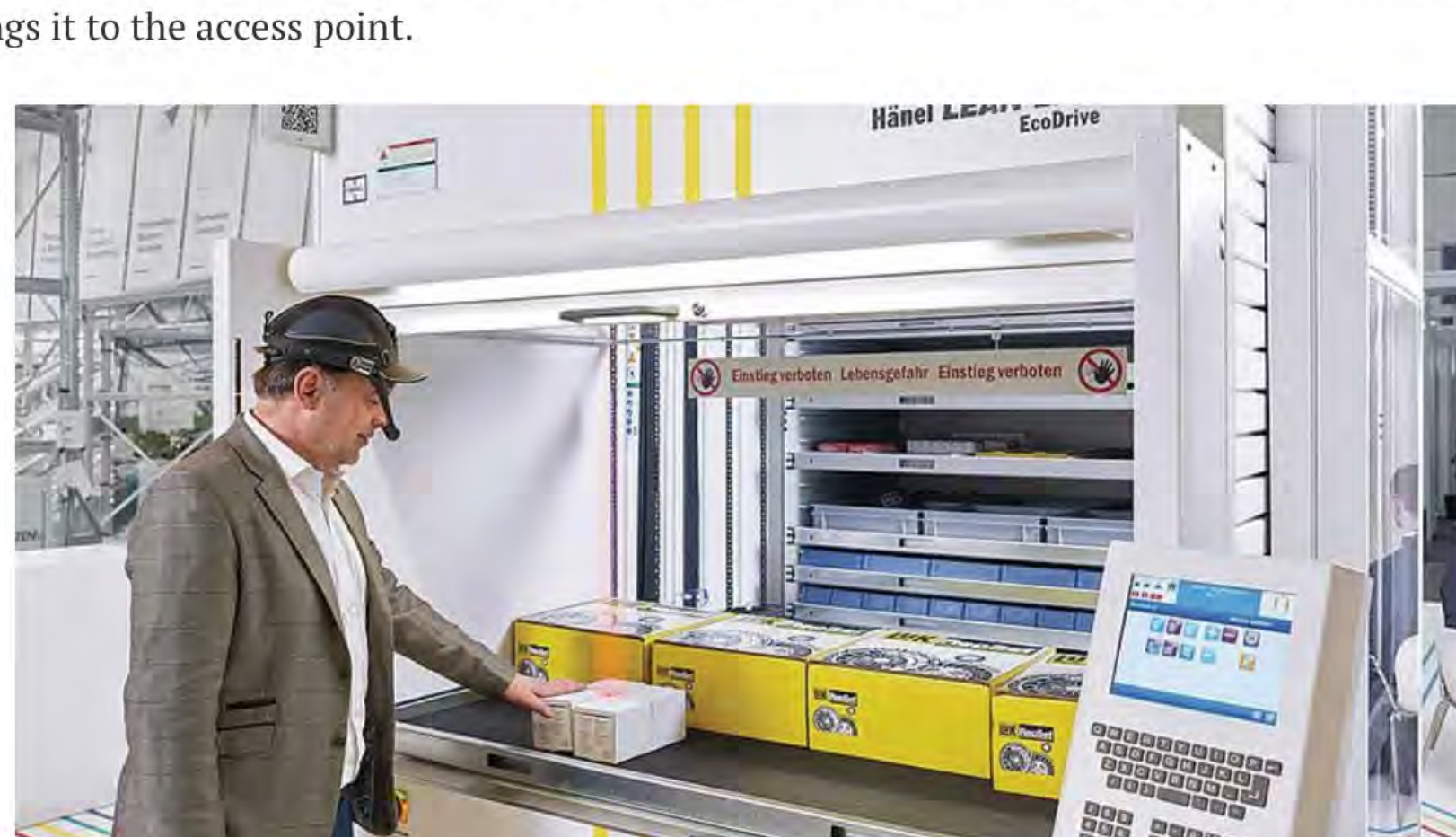
Hanel Storage Systems collaborated with IT specialists at MAN to link two Hanel Lean-Lift systems to SAP and enable storage system operation via smartglasses.
