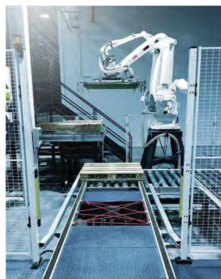
Viastore introduced fully integrated refrigerated and frozen pallet AS/RS for production, distribution and 3PL support, including automated layer picking, semi-automated individual case picking and automated transport to the shipping dock.
